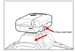
To remove the flash trigger, press and hold the release button and slide it out from the camera.
