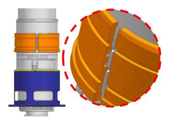
3. Insert the focus c-ring as shown and place it over the lens Make sure the flange of the c-ring downwards
