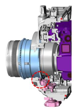
The Canon RF 15-35 mm F/2.8L IS zoom gear can be controlled by zoom of the housing; The Canon RF 24-70 focus gear can be controlled by extension ring with focus knob After mount the camera and lens (with gear installed) on the housing, confirm that the zoom and focus operates correctly.
