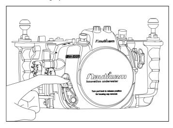
Push the safety button of the port locking lever downwards.
