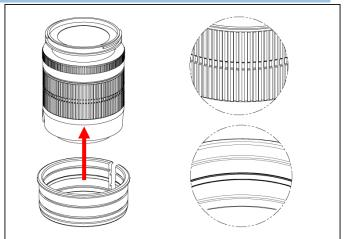
Insert the plastic c-ring as shown and place it over the lens rubber zoom ring.
