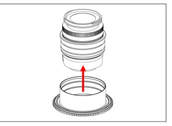
Insert the gear on the plastic c-ring until it reaches the flange of the plastic c-ring.
