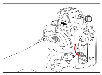
Lock the port into place by turning the port locking lever to the inward position. To ensure that the port is securely mounted, confirm that the green line on the safety button of the port locking lever is visible.
