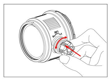
Engage the gear by pushing in the knob, then turn the knob both ways to check if the lens focuses.
