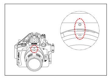
Align the Port mounting indices of the port and the housing.
