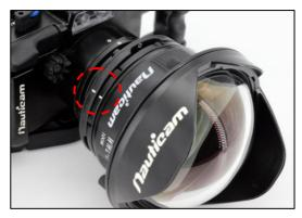
2. Remove the lens when "I" mark on the lens aligns with the "I" mark Bayonet Mount.
