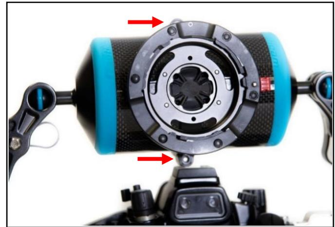
Align the bayonet holder by the screw holes, and secure the bayonet holder by tightening the 2x screws
