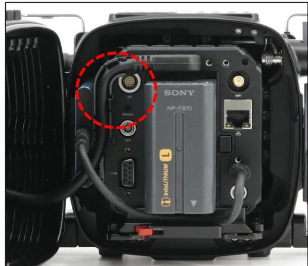
Connect the HDMI 2.0 cable through the camera's HDMI port as shown. The clamp is used to avoid over bending or twisting the cable and extend the cable's lifecycle.
