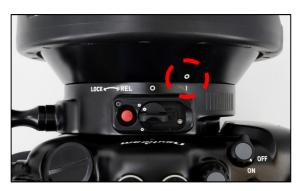
4. Align the "I" mark on the adaptor with the WHITE dot on the port. Gently push the port towards the adaptor until it cannot go in any further.
