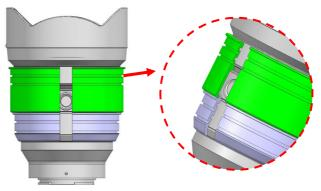
2. Insert the plastic C-ring for focus as shown and place it over the lens, then lock the focus c-ring as shown.
