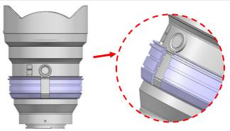
Insert the plastic C-ring for zoom as shown and place it over the lens
