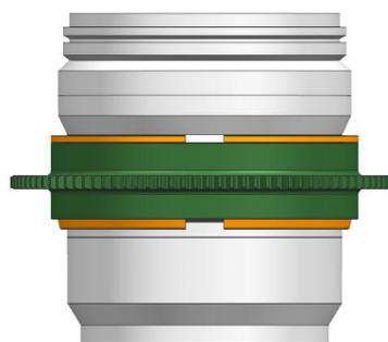
3. To remove the PL2060-Z Zoom Gear, reverse the above steps. The tightness between the PL2060-Z Zoom Gear and the lens can be adjusted by removing or adding rubber grips on either sides of the plastic C-ring, spare rubber grips are included in the package.
