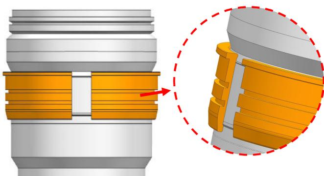
1. Insert the plastic C-ring as shown and place it over the lens
