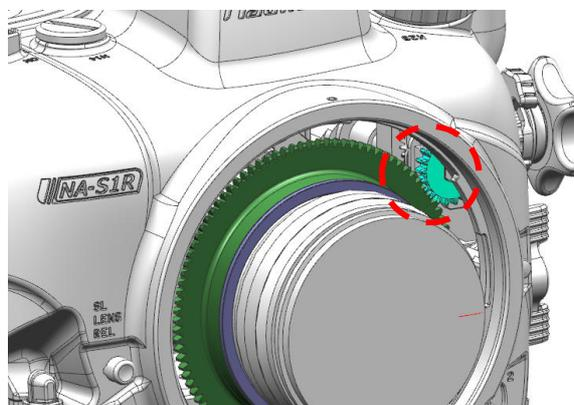
1. The PL2060-Z Zoom Gear can be controlled by zoom/focus knob of the housing.
