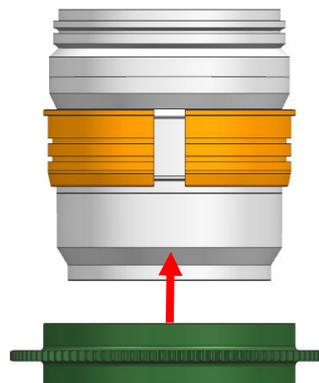
2. Insert the PL2060-Z Zoom Gear on the plastic C-ring until it reaches the flange of the plastic C-ring.
