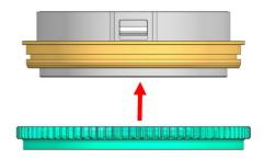
Insert the gear for Canon EF-EOS R Control Ring Mount Adaptor on the plastic C-ring until it reaches the flange of the plastic Cring.
