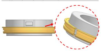
1. Insert the plastic C-ring as shown and place it over the adaptor
