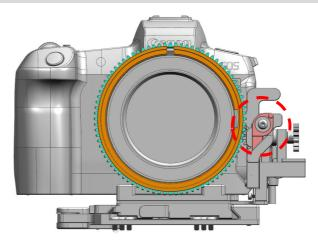
Before mount the camera and adaptor (with gear installed) on the camera tray, make sure the marked/highlighted lever is downward as shown.
