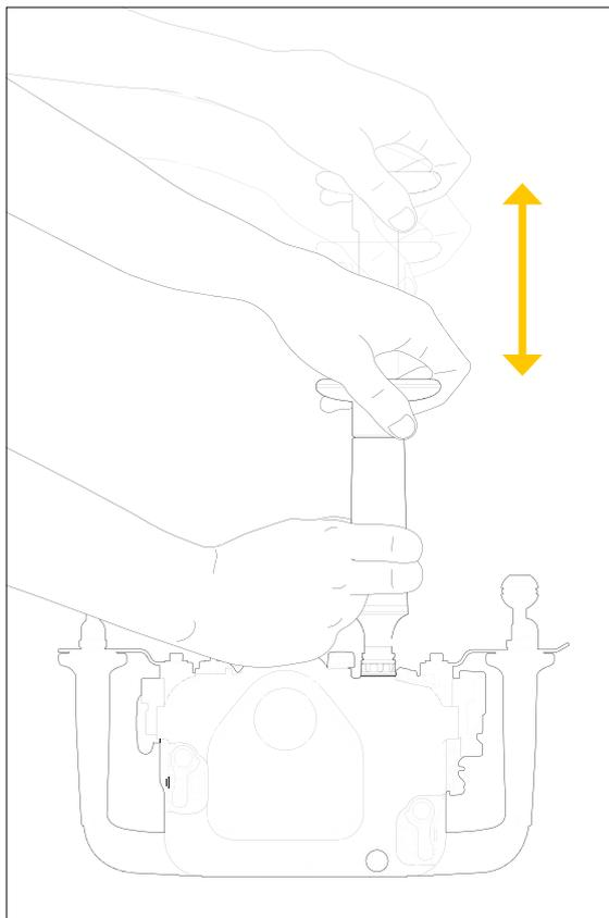
connect hand pump to the valve and pump several times until it reaches the target vacuum level
