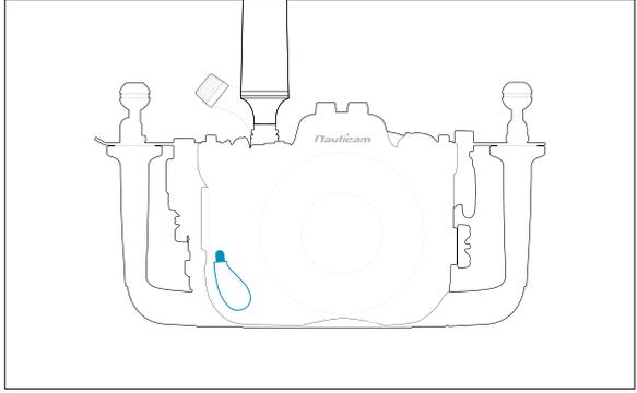
reset vacuum valve system using hand pump then close the cap
