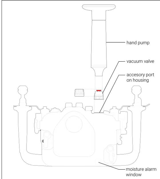
remove the plug of M16 accessory port from the housing
