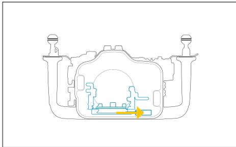
unlock camera tray lever and remove the tray from the housing
