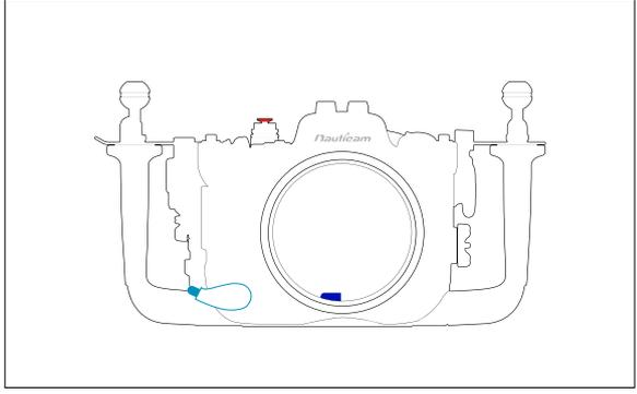
press the blue button to reset vacuum alarm before replacing port
