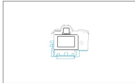
attach the camera tray by tightening the tray screw into the tripod socket of the camera
