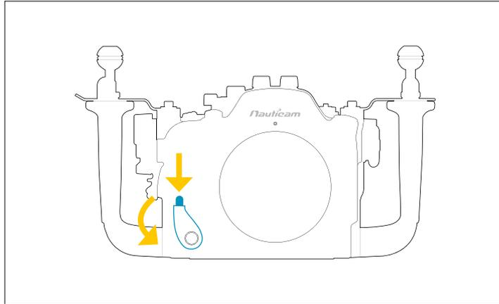
depress safety button and rotate anti-clockwise
