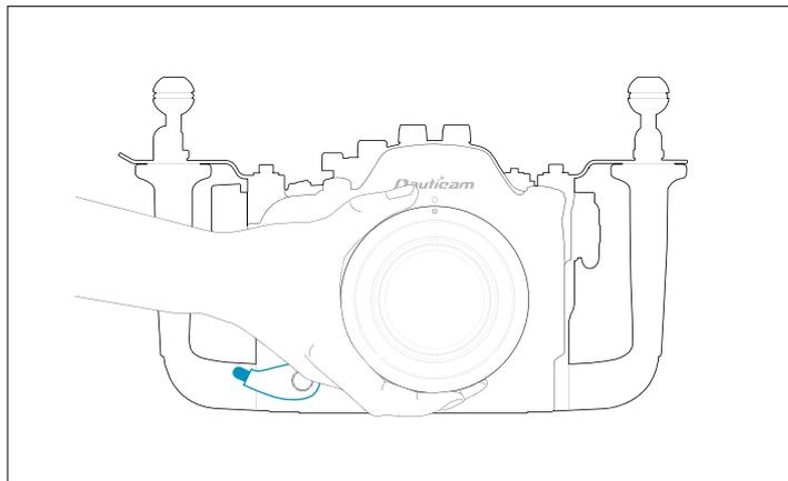
lubricant the port O-ring before mounting
