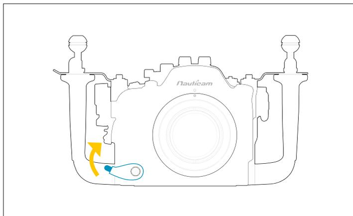
rotate locking lever clockwise to lock
