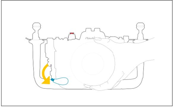
unlock port lock and remove port assembly
