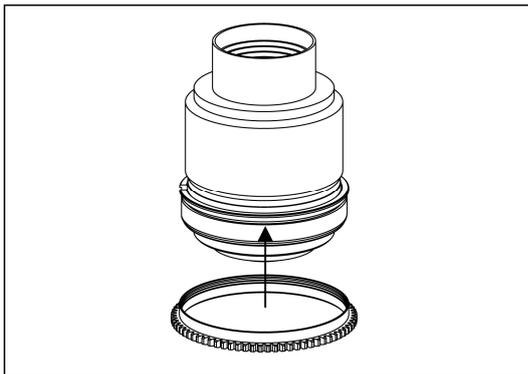
2. Insert the gear of X60-A on the plastic c-ring until it reaches the flange of the plastic c-ring.
