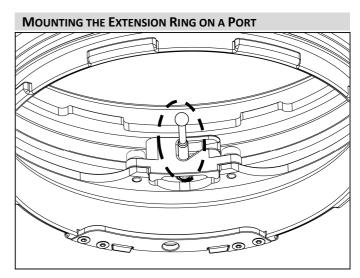
Confirm that the extension ring is unlocked, with the locking pin pointing upwards as shown.
