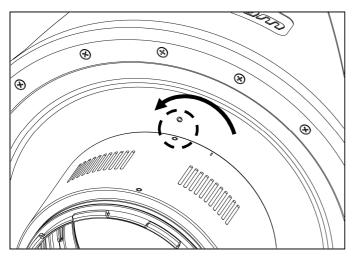
Turn the extension ring clockwise until the white dot on the extension ring aligns with the white dot on the port.
