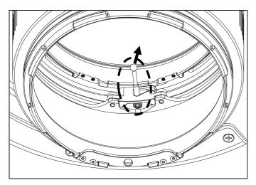
To lock the extension ring, push the locking pin inwards.
