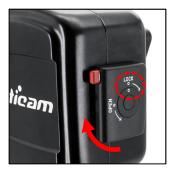
4. Turn the housing lock 270° clockwise until the lock reaches the "lock" position as shown. Confirm that the white indicator line on the safety button is visible.
