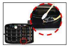
3. Test the alarm by connecting the two wires near the bottom of the housing with a damp cotton bud; the alarm should start giving out a repeating "beep" sound along with a flashing red light. The "beep" sound and the light should keep on going for 5 seconds after the removal of the damp cotton bud.
