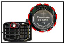
Ensure that remove an insulation film before install a battery.
