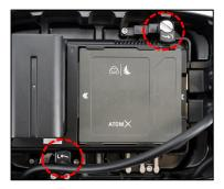
Secure the monitor by turning the two locking levers towards the monitor as shown.
