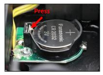
To remove the battery, press the metal plate as indicated and the battery will pop out.
