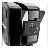
Close the housing while the housing lock is in the "Open" position.
