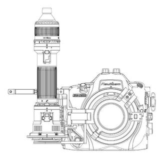
3. Mount the EMWL focusing unit on the EMWL holder as shown.
