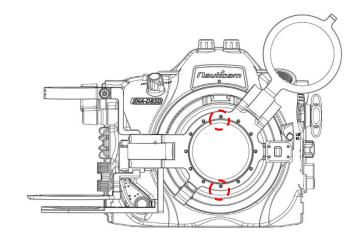
2. Align the two positioning screws on the back of the holder with the slots on the front of the port.
