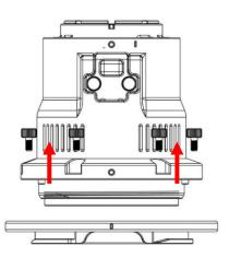
1. Remove a bayonet mounting ring from EMWL focusing unit by unscrewing 6x thumb screws as shown.
