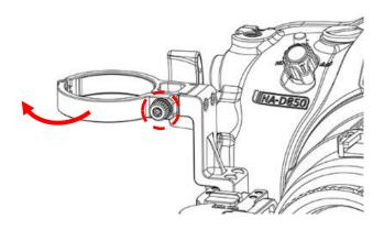
2. Open the relay lens holder by unscrewing the thumb screw.
