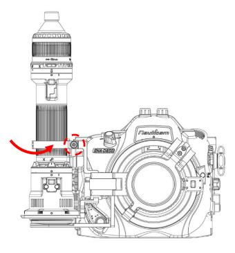
5. Close the relay lens holder and securely tighten with the thumb screw.
