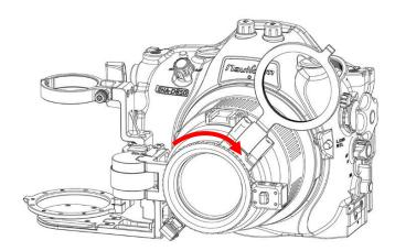
3. Fasten the holder by screwing the locking ring into the thread on the front of the port.
