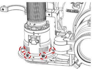
4. Secure the EMWL on the flip holder by tightening 6x thumb screws.
