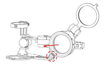
1. Press the lever for diopter holder and open the diopter holder to the side then remove the locking ring from the flip holder.
