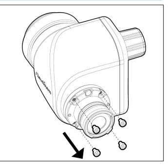
Unlock and remove the four S.S. screws from viewfinder body as shown.
