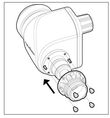
Align the two pins on the viewfinder body, and install the collar adaptor by tightening four S.S. screws provided.
