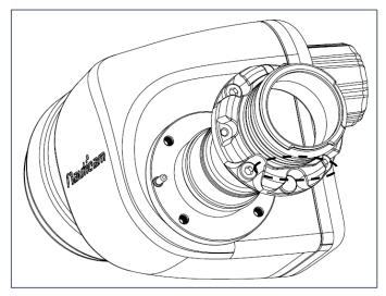
Align the adaptor groove as shown above, make sure it is facing downwards while installing the adaptor into the viewfinder.
