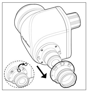
Remove the two screw cap covers, and install one of the existing screws to push and separate the collar from the viewfinder body.
