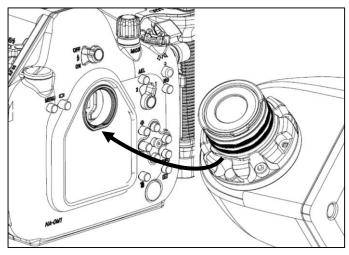
Remove the retainer O-ring of the viewfinder, and align the viewfinder groove with the sleeve in the display window as shown.
